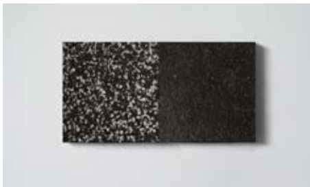
Figure 1b: Recycled Polyurethane Foam & Shanxi Black Granite. FOAM STONE CAFE S U G I B E R R Y 2016, Kortrijk (BE)
